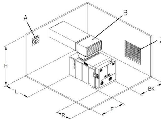
Recommended machine placement and dimensions
